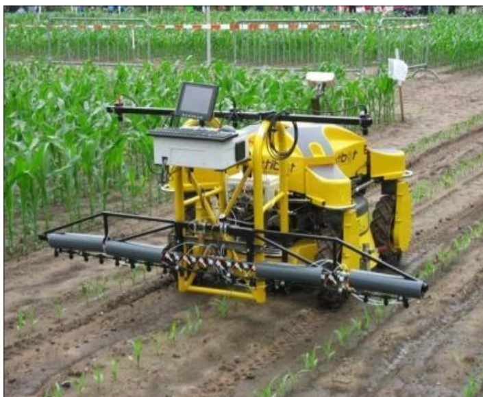
‘Hortibot’, an example of high-tech precision spraying machinery. © Aarhus University, Denmark.
